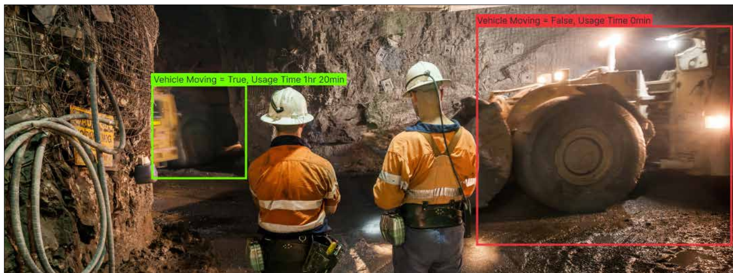
alwaysAI's computer vision can detect and track vehicle movement inside a mine. Image courtesy of alwaysAI
